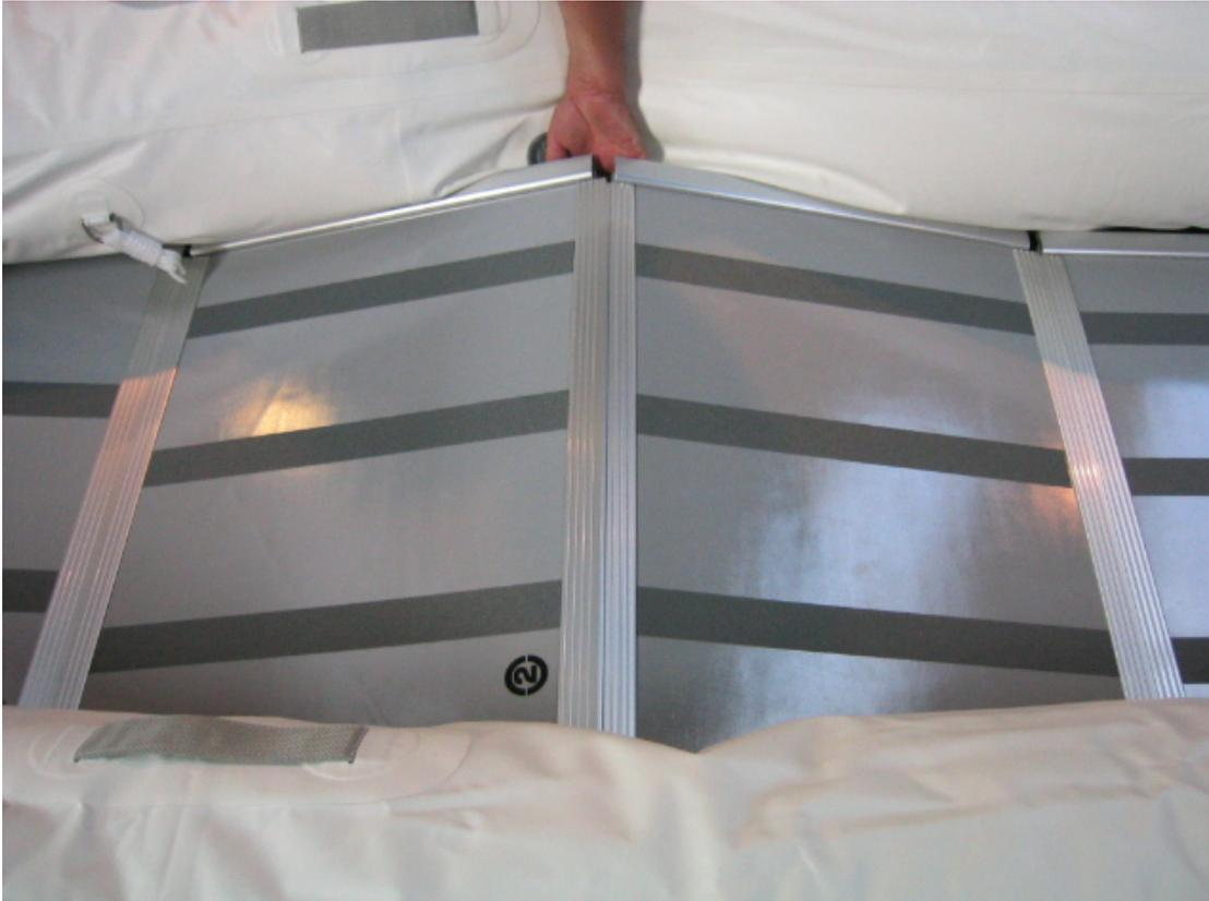
3. Press the ridge down until all the boards are flat, making sure you haven't trapped any of the pontoon fabric or valve bungs (including the keel valve) underneath. Check all boards are in line still. If you have difficulty at this step you probably have too much air in the pontoons still, or you have some of the pontoon fabric pinched under the boards.
